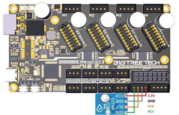
3.5. I2C (e.g., AHT10 Temperature and Humidity Sensor) Wiring
